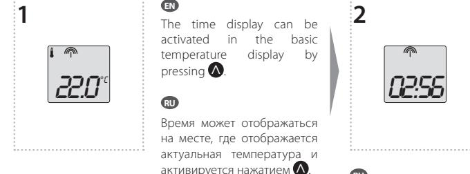
**EN** The time display can be activated in the basic temperature display by pressing .
