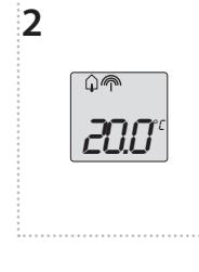
**EN** Press the button or to display the set temperature (if the display backlighting is activated, the first press of the button illuminates the backlighting and the second press switches the display). The displayed value flashes. Press to set the required temperature.
