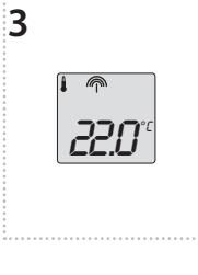
**EN** 5 seconds after the last pressing of the button, the display of the set temperature switches back to the current temperature - the value is saved in the memory.
