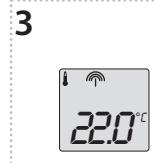
**EN** 5 seconds after the last pressing of the button, the display of the set temperature switches back to the current temperature - the value is saved in the memory.
