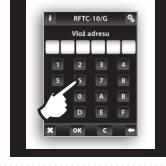
**EN** On the control unit, enter the address of OPT-RFTC-111 (see manual of control unit).
