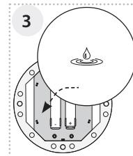
**EN** Replace the seal, attach the front cover - make sure the correct location. Screw in, tighten the screws to maintain IP protection.
