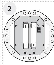
**EN** Replace the batteries and check the correct location (when the batteries are inserted, the blue LED lights up for 2 seconds and a message is sent to the device at the same time).
