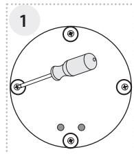
**EN** Use a screwdriver to open the detector.
